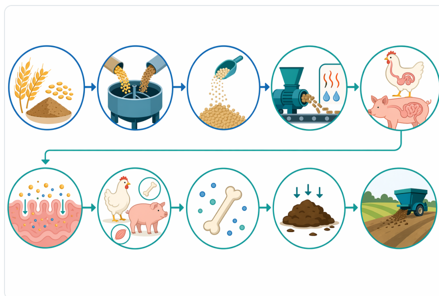
Figure 2. Thermostable phytase is intended to survive conditioning, pelleting, or extrusion so active enzyme remains available for phytate hydrolysis after ingestion.
