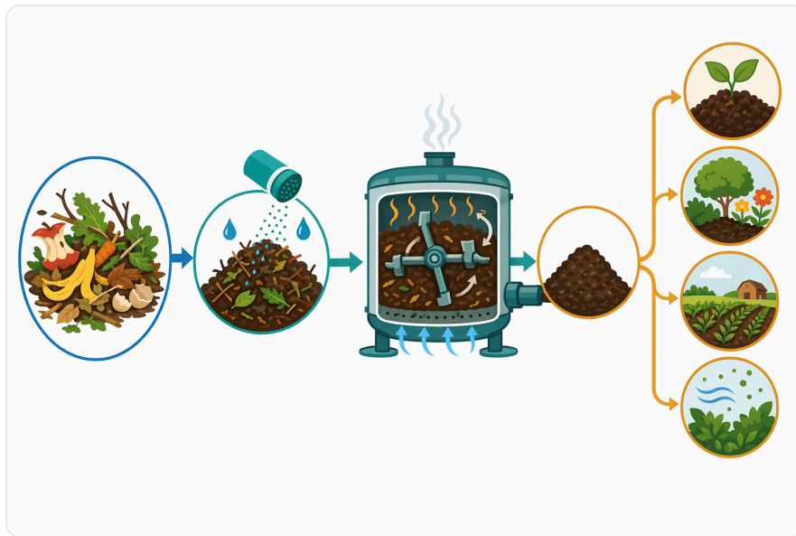
Figure 2. A solid-waste bacterial treatment is typically dosed into moist, aerated organic waste to accelerate stabilization and compost formation.
