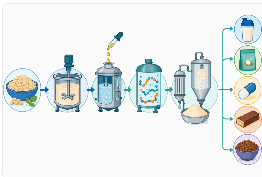
Figure 8. A controlled soy peptide process typically disperses the substrate, adds protease under suitable conditions, stops hydrolysis, and then clarifies, concentrates, dries, blends, or further processes the hydrolysate.
