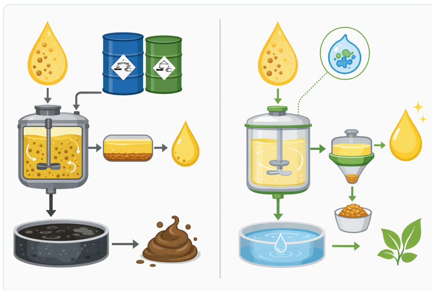
Figure 4. Compared with chemical degumming, enzymatic phospholipase treatment can increase oil yield and reduce chemical load and wastewater.
