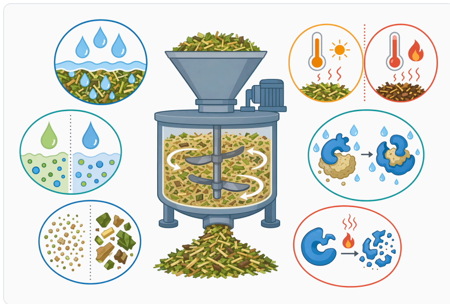
Figure 7. Moisture, heat exposure, pH environment, particle size, and mixing all influence whether pectinase can contact pectin and remain functional.
