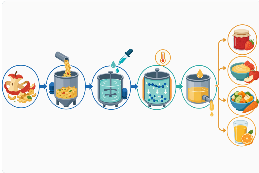
Figure 2. Industrial PME processing converts native pectin in fruit materials into controlled low-methoxyl pectin functionality for texture, clarification, and gel formation
