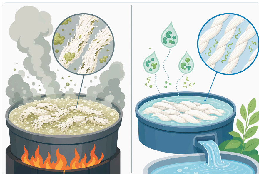
Figure 4. Compared with conventional alkaline scouring, pectate lyase bioscouring can lower chemical severity while preserving fiber quality.
