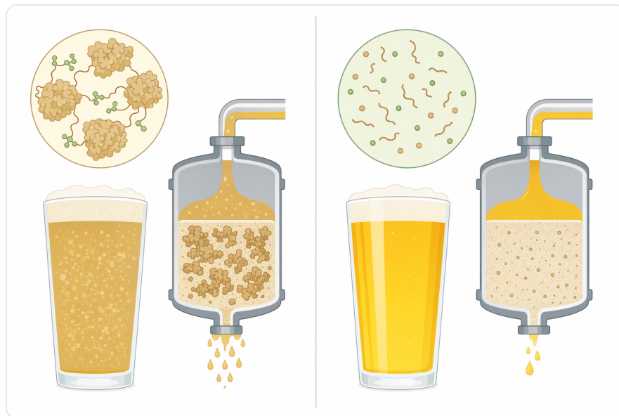
Figure 4. Papain provides broad plant-derived proteolysis, while proline-specific endoproteases and non-enzymatic adsorbents address beer stability through different target selectivity or removal mechanisms.
