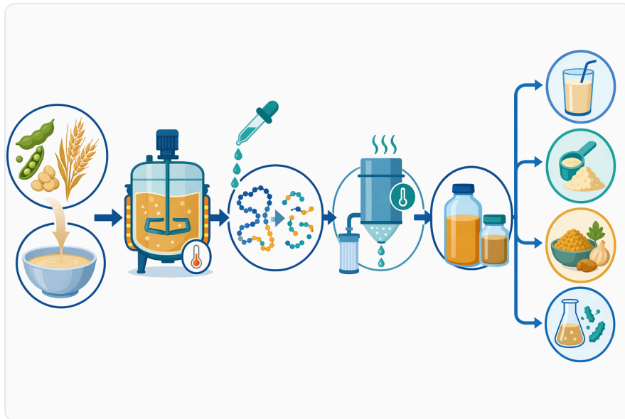
Figure 7. A typical papain hydrolysis process hydrates the plant protein, adds enzyme, controls contact time, inactivates the reaction, and then blends, heats, dries, or formulates the hydrolysate.
