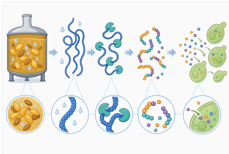
Figure 3. Neutral protease increases yeast-available nitrogen by converting larger grain proteins into amino acids and short peptides that can support fermentation.
