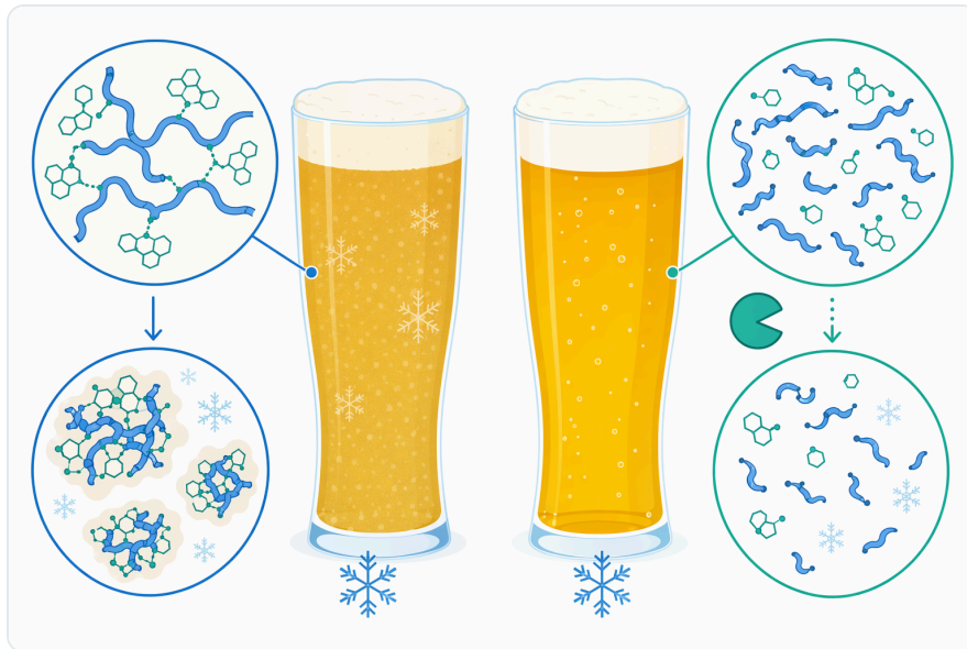
Figure 4. By reducing the size and cross-linking capacity of susceptible protein fractions, mash-stage protease treatment can help lower the pool of material involved in protein-polyphenol haze.
