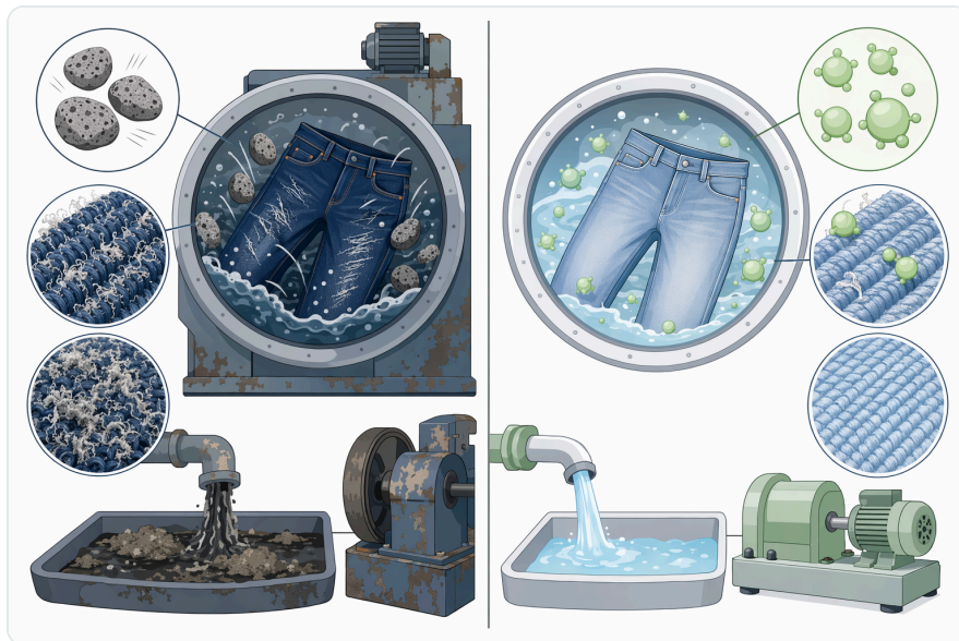
Figure 4. Compared with pumice-only abrasion, neutral cellulase denim washing gives more controlled fading with less fabric damage and lower solid waste.
