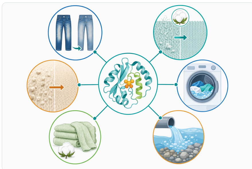
Figure 3. Neutral cellulase is used in denim fading, cotton bio-polishing, defuzzing, anti-pilling, and garment softness improvement.
