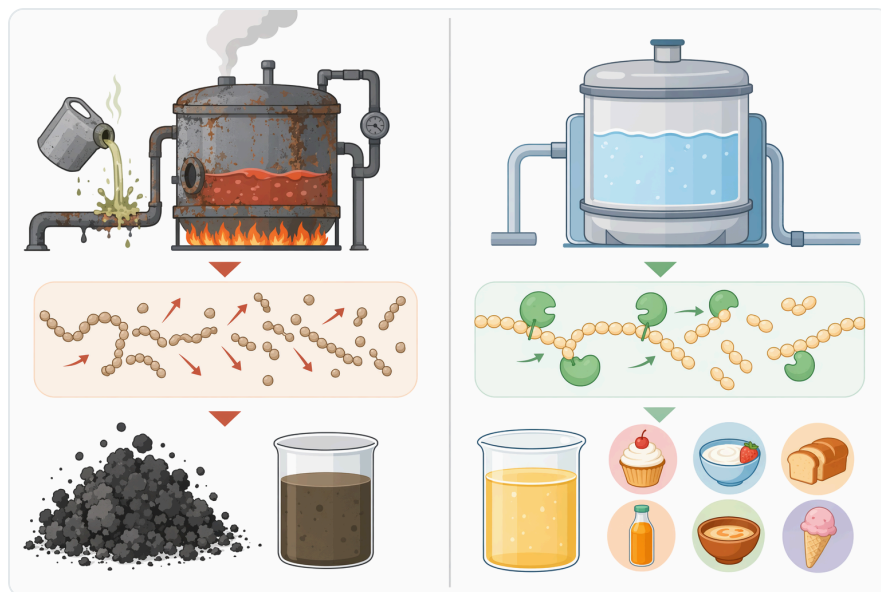
Figure 4. Compared with acid starch hydrolysis, alpha-amylase liquefaction offers milder processing, more controlled dextrin formation, and fewer undesirable byproducts.
