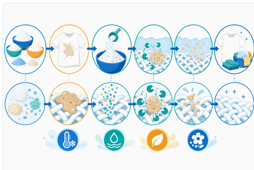
Figure 5. In a wash cycle, water hydrates the gum stain, mannanase diffuses into accessible regions, polymer chains are cleaved, and the detergent system disperses the loosened residue.
