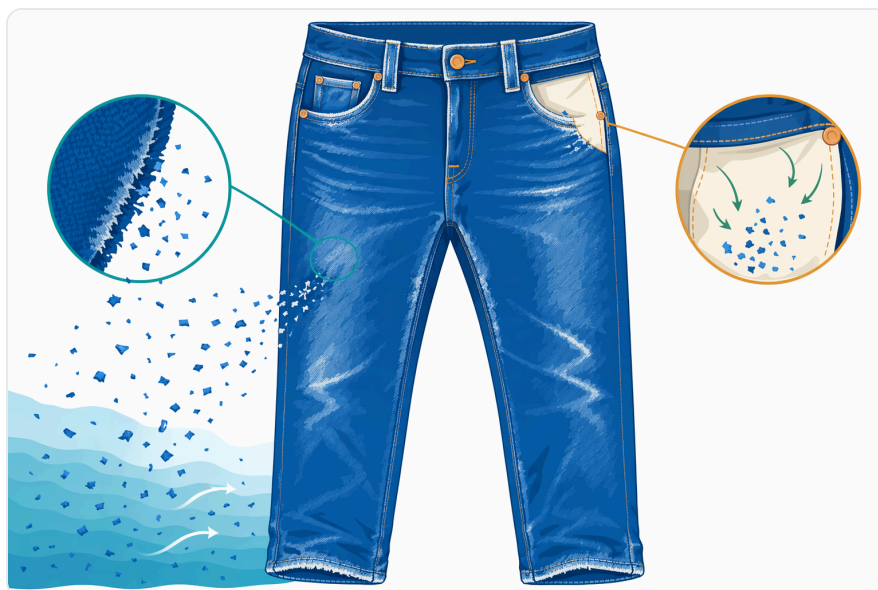
Figure 3. Visible denim wash-down appears first on exposed high-friction zones where loosened fibrils and indigo-bearing fragments detach most readily.
