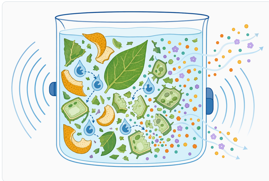
Figure 5. Pectinase-assisted extraction improves release by weakening pectin-rich cell-wall barriers while physical mixing or ultrasound improves mass transfer.
