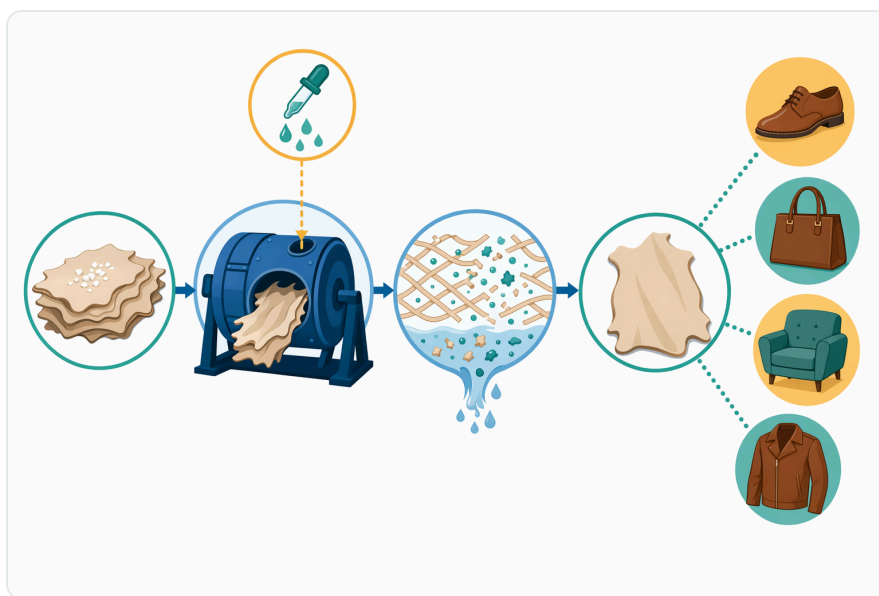
Figure 3. Controlled hydrolysis can progress from peptide-bond cleavage to reduced protein barriers, improved fiber opening, better chemical diffusion, and more uniform leather properties.
