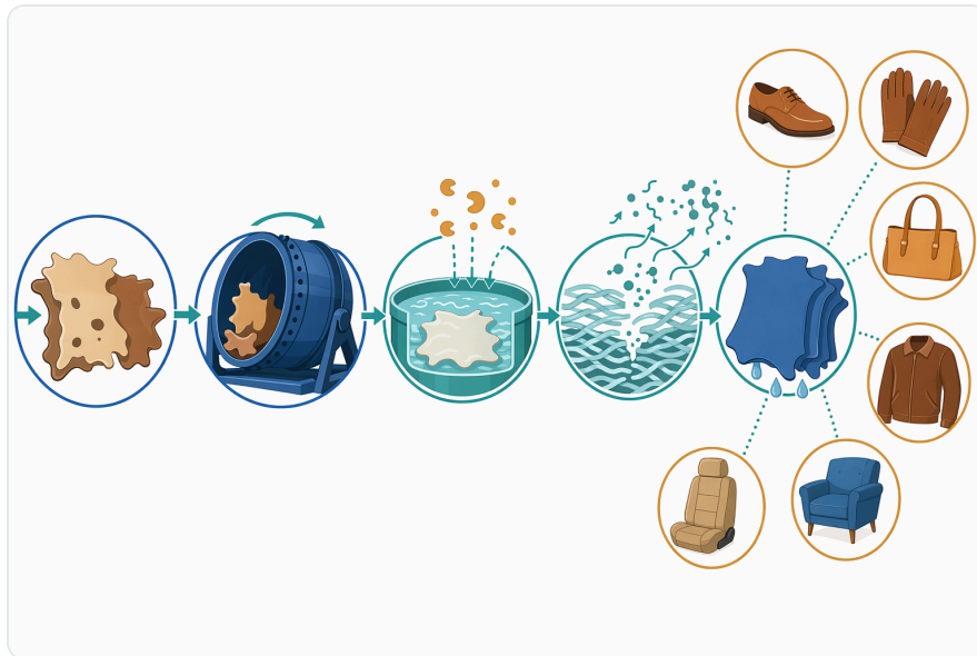
Figure 3. Trypsin bating is positioned after liming and deliming and before pickling, tanning, and post-tanning operations.
