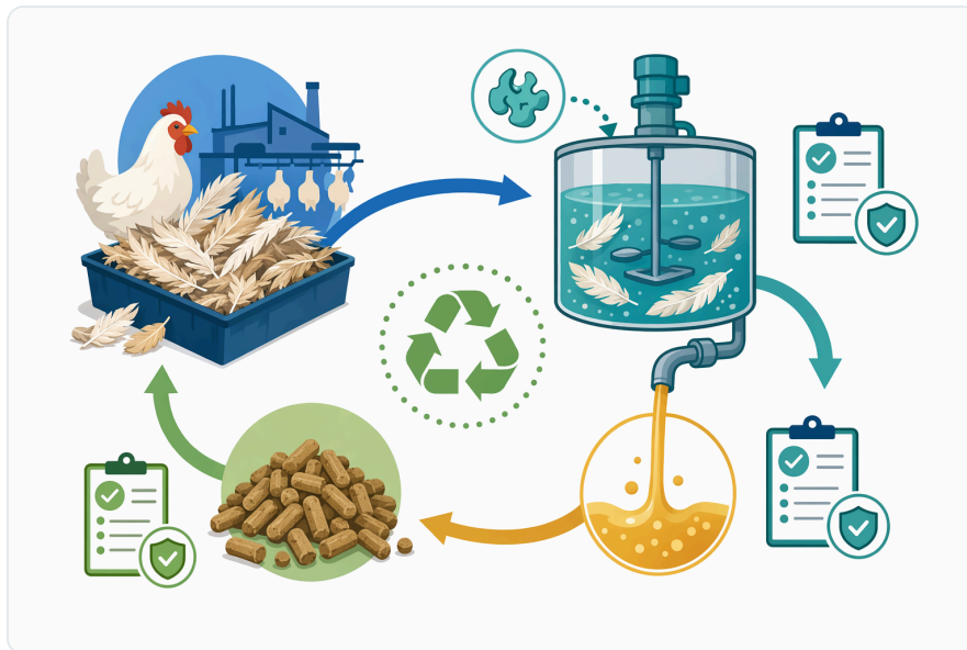
Figure 7. Keratinase supports by-product valorization by converting feather waste into a more usable protein hydrolysate when safety, quality and formulation requirements are met.
