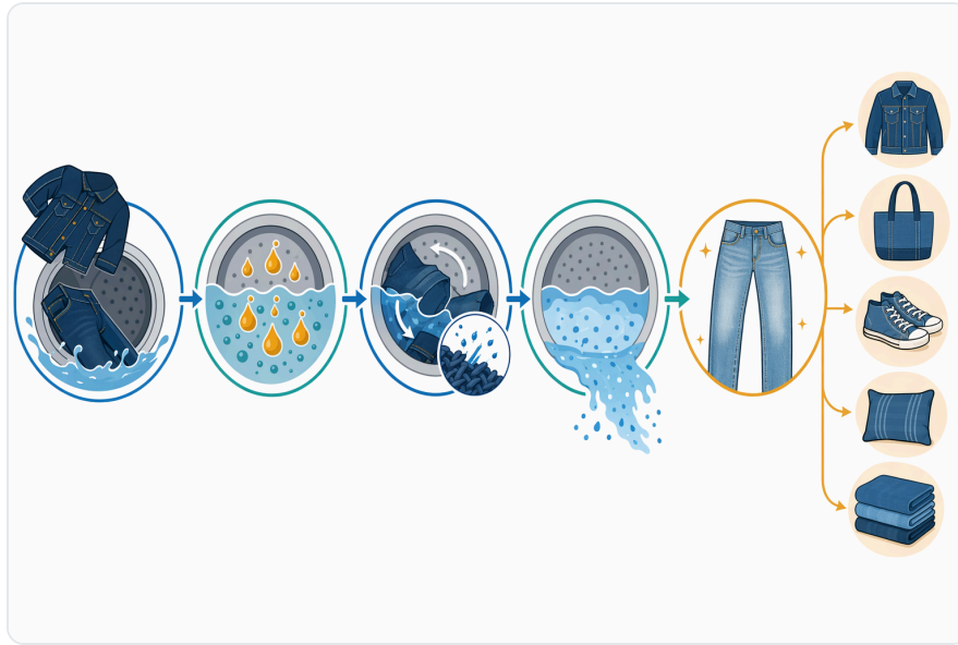
Figure 4. Backstaining occurs when released indigo particles are not kept dispersed and rinsed away before they redeposit on lighter denim areas.
