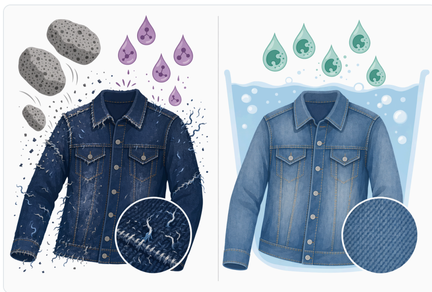
Figure 3. Cellulase-based fading removes dye-bearing cotton surface material, whereas laccase-type decolorization acts through oxidative changes to susceptible dye chromophores.
