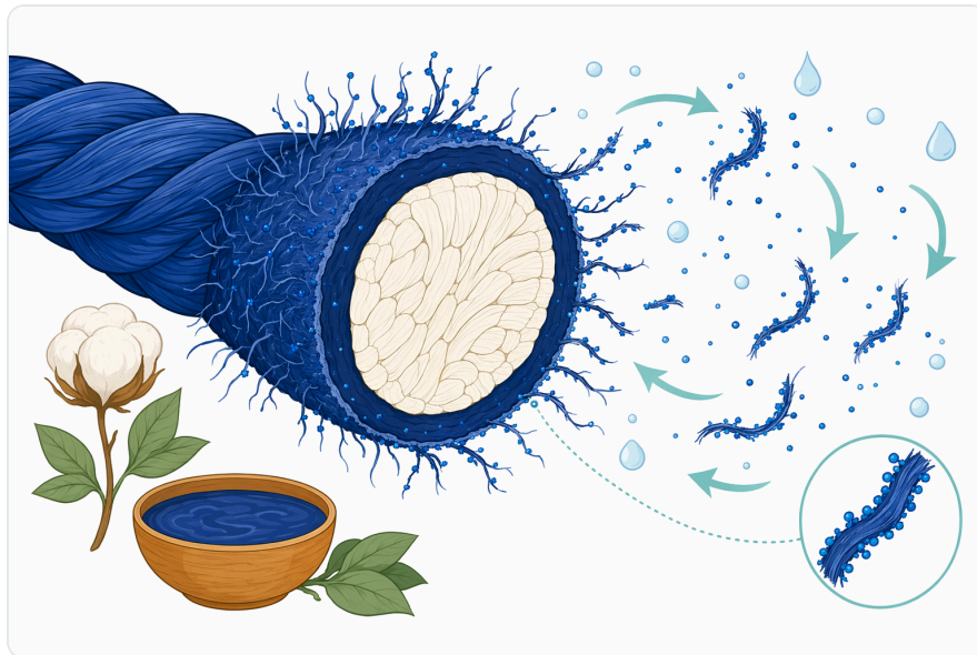
Figure 1. Indigo fading in enzyme denim washing is mainly a surface effect because much of the visible blue color is concentrated near the yarn exterior.
