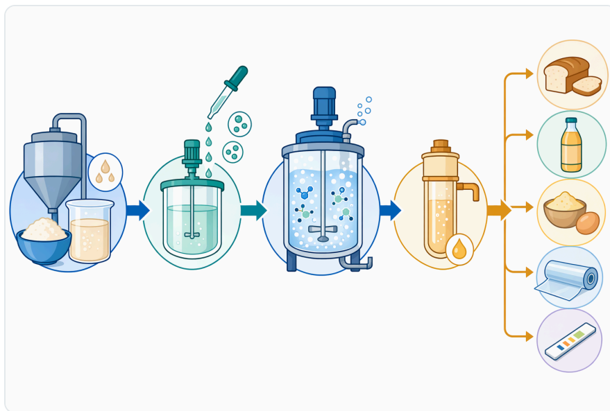
Figure 2. Industrial glucose oxidase workflows combine controlled dosing and aeration to generate oxygen-scavenging or oxidative effects in foods and diagnostics.
