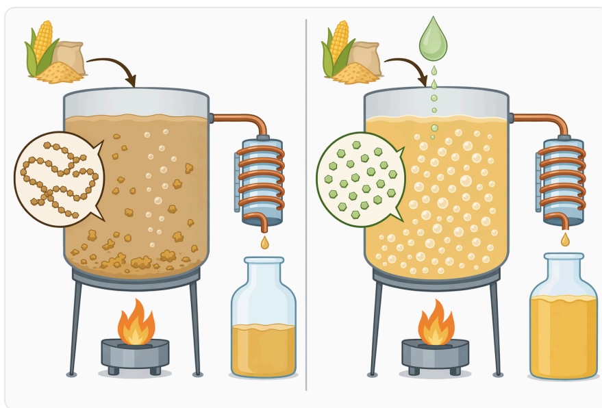
Figure 4. Compared with relying on malt enzymes alone, added glucoamylase increases glucose release, attenuation, and final fermentable yield from starch-rich mash.
