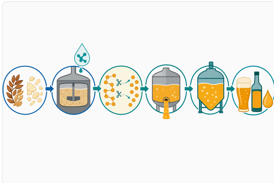
Figure 2. In brewing and distilling, liquid glucoamylase is dosed into mash or wort to drive starch conversion toward highly fermentable sugars.
