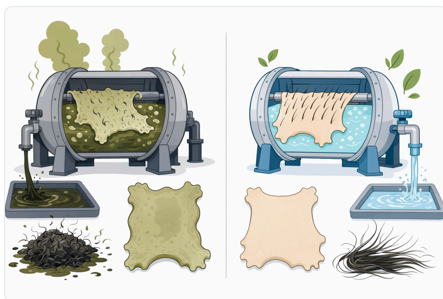
Figure 3. Lime–sulfide dehairing primarily attacks keratin and can pulp hair, whereas enzyme-assisted dehairing focuses on weakening the hair anchoring environment.
