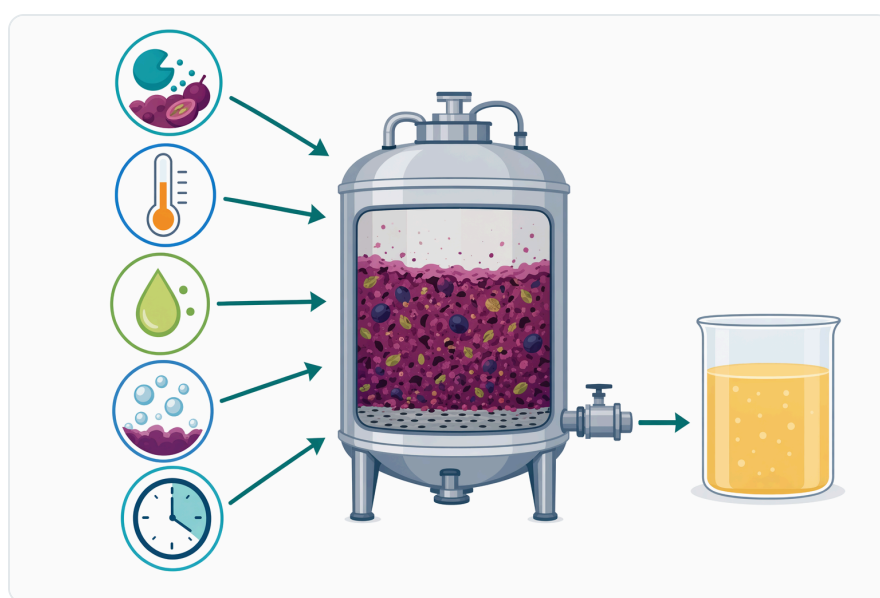
Figure 7. Pectinase performance depends on contact with accessible pectin, processing order, temperature, acidity, alcohol environment, and reaction time.
