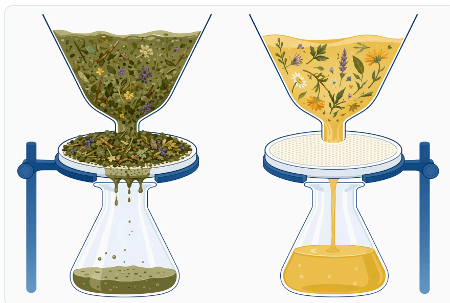
Figure 4. By shortening pectin chains, pectinase can improve clarification and reduce filtration resistance in pectin-rich botanical liquids.
