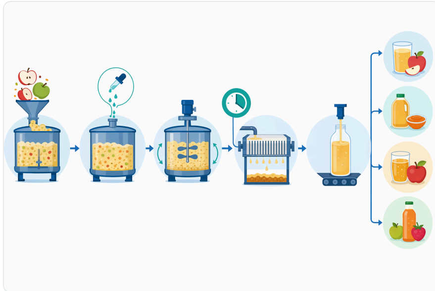
Figure 2. In apple processing, pectinase is added after crushing to reduce viscosity, improve juice release, and accelerate filtration.
