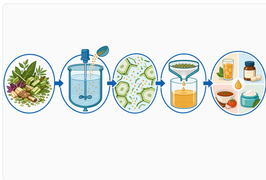
Figure 8. A typical enzyme-assisted extraction sequence adds \beta -glucanase during an aqueous maceration, steeping, slurry-holding, or extraction step before clarification and downstream finishing.
