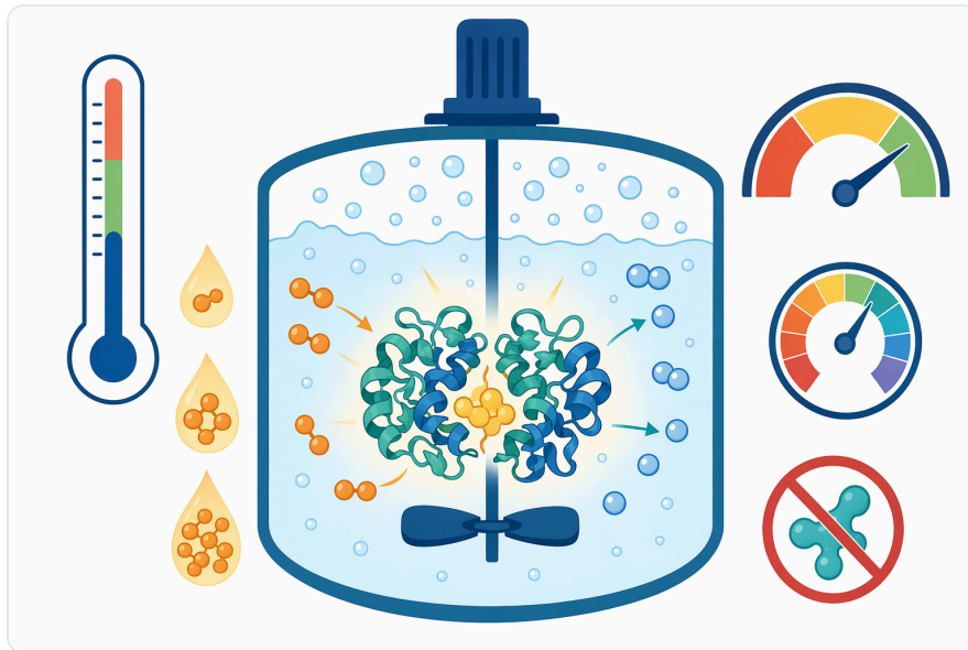
Figure 6. Catalase performance depends on enzyme-compatible conditions including temperature, pH, mixing, peroxide exposure, and inhibitors.
