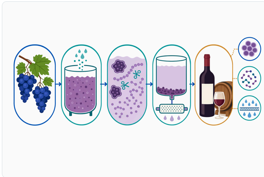
Figure 7. \beta -Glucanase fits as a process step before clarification or filtration, or during planned lees contact when glucan-containing substrates are present.
