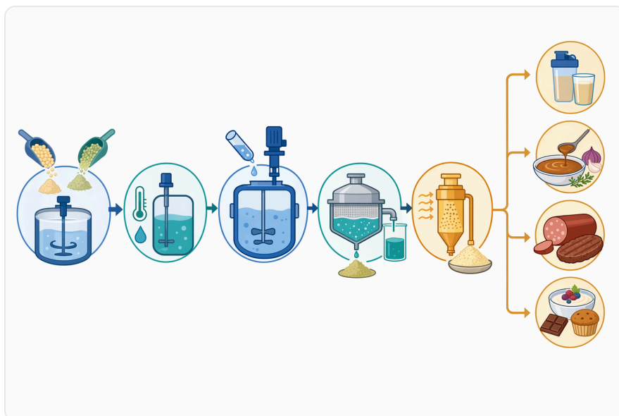
Figure 6. A typical alkaline protein hydrolysis process includes substrate hydration, pH adjustment, enzyme addition, time-temperature control, endpoint selection, enzyme inactivation, and downstream handling.
