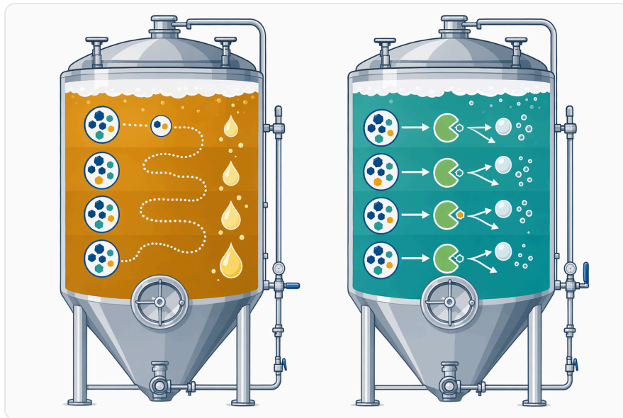
Figure 4. Brewing studies support using ALDC activity during fermentation to reduce the pathway that leads to diacetyl.
