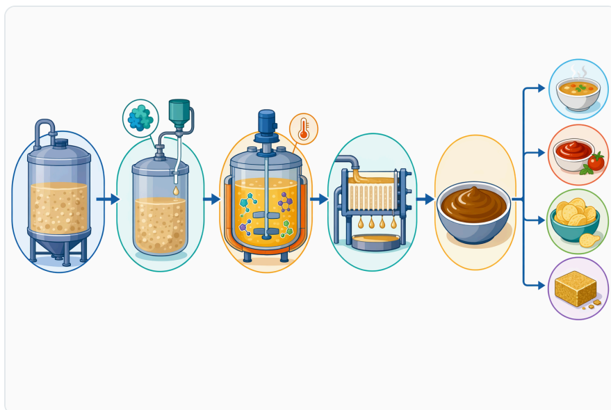
Figure 2. A typical process adds deaminase to yeast extract under mild heat and pH control before finishing the umami-rich seasoning ingredient.
