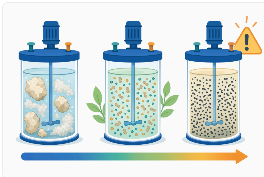
Figure 3. Hydrolysis depth must be controlled because limited, optimized, and excessive cleavage can produce different solubility and flavor outcomes.
