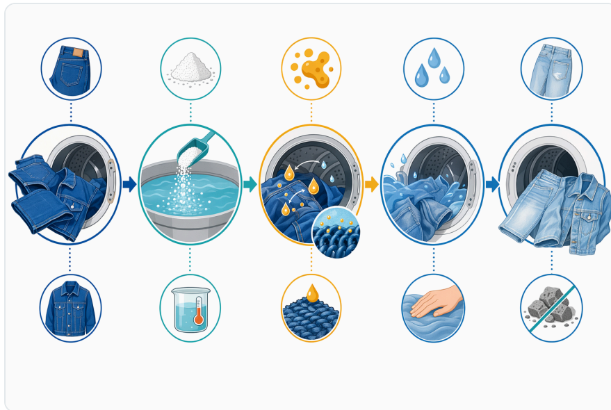
Figure 5. A cellulase stone wash is a wet mechanical sequence in which enzyme contact, tumbling, removal of loosened material, stopping, and rinsing must be controlled.
