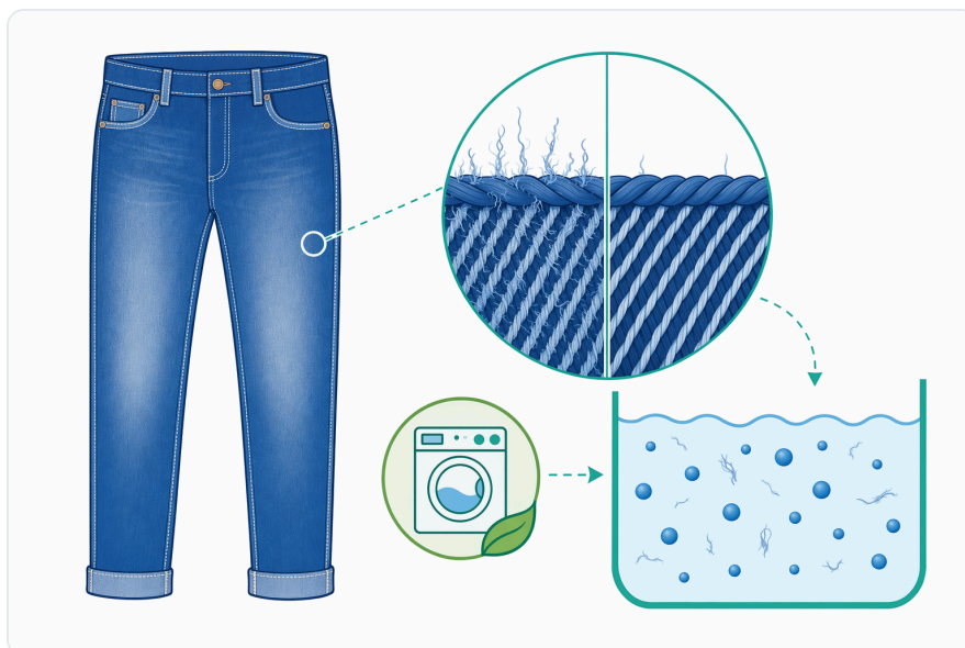
Figure 4. Enzyme stone washing can reduce exposed-area shade, lower surface fuzz, soften the hand, and release dye-containing fines into the bath.
