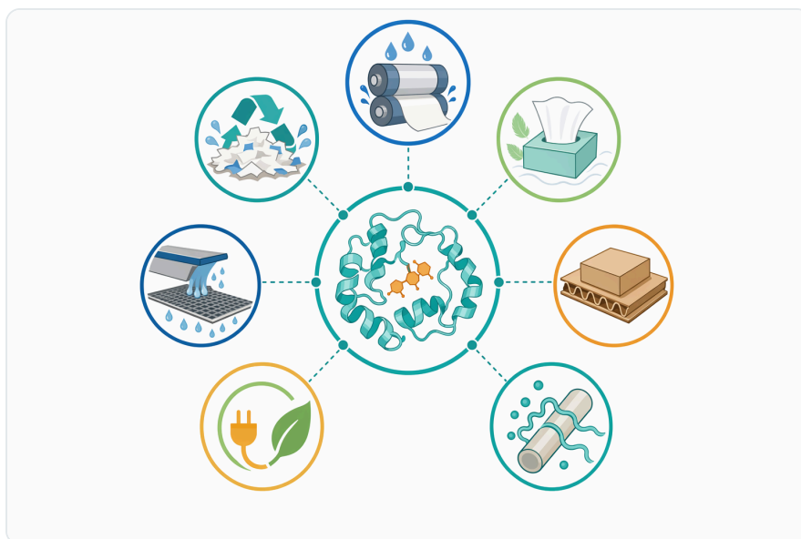
Figure 5. Cellulase applications in paper and pulp include deinking, white-water fines control, drainage support, refining aid use, biobleaching support, nanocellulose production, and sludge valorisation.
