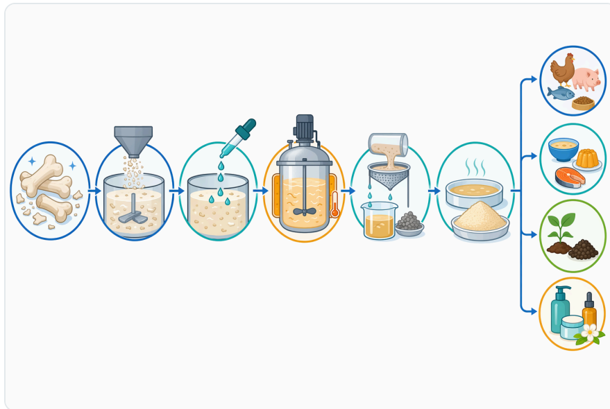
Figure 3. Substrate preparation steps such as size reduction, heating control, degreasing, and optional demineralization improve the accessibility of bone protein to protease action.
