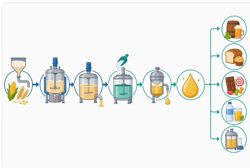
Figure 6. In brewing and distilling, starch opening, alpha-amylase liquefaction, beta-amylase maltose formation, and yeast fermentation act as linked process stages.
