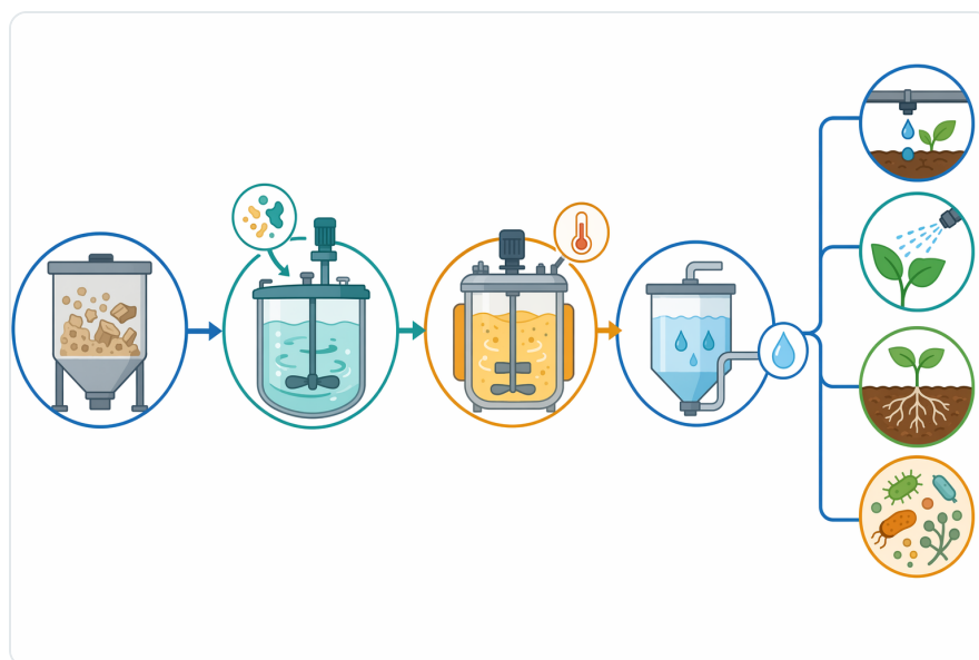
Figure 3. Aqueous enzyme treatment can convert selected organic nutrient fractions before mineral and amino-acid components are finalized into a water-soluble fertilizer blend.
