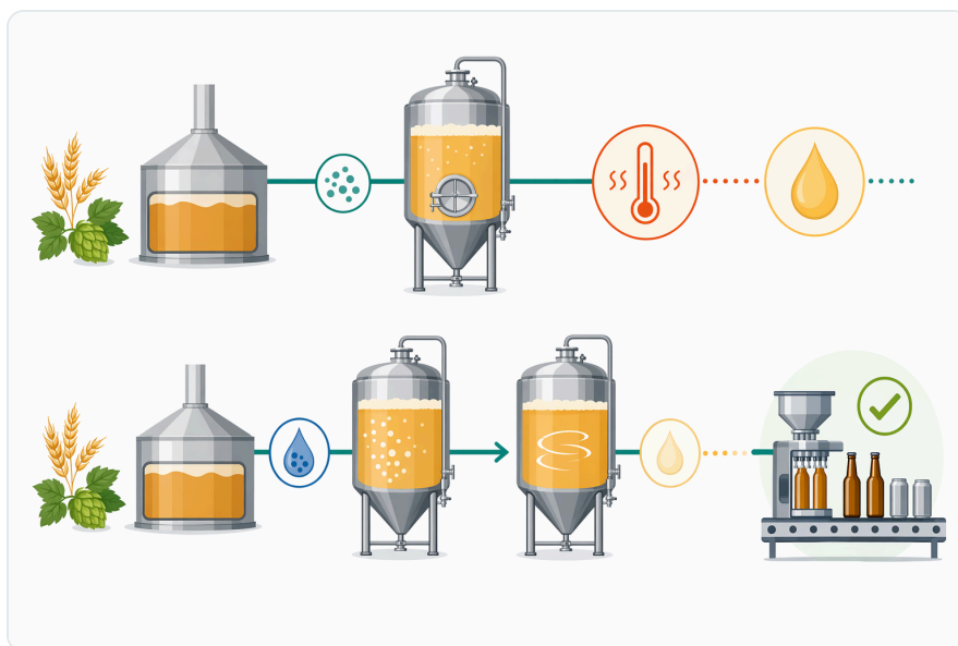
Figure 5. By reducing diacetyl formation, ALDC can make maturation less dependent on an extended late-stage cleanup period.
