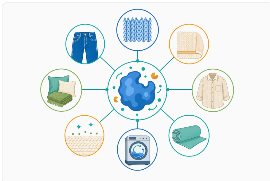
Figure 3. Acid cellulase is used across cotton bio-polishing, anti-pilling treatment, denim washing, linen softening, and preparation of cellulosic surfaces for later finishing.
