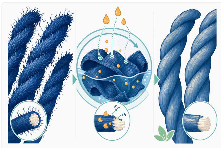
Figure 6. In denim and cotton finishing, acid cellulase acts mainly on exposed surface fibrils when treatment is controlled.
