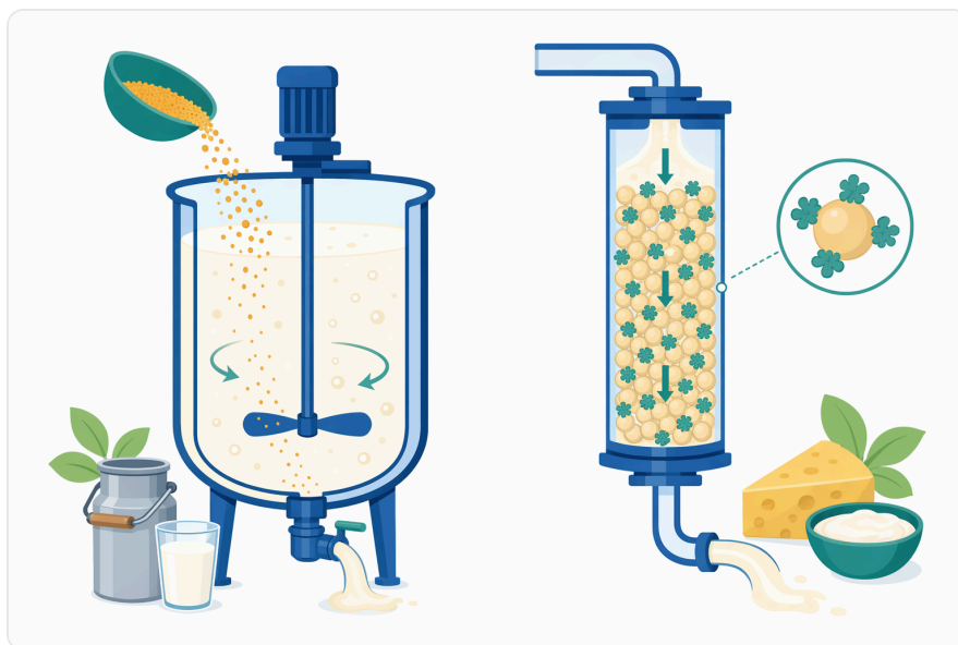
Figure 6. Soluble lactase powder is used by direct addition, whereas immobilized lactase systems retain the enzyme on a support for reuse or continuous processing.
