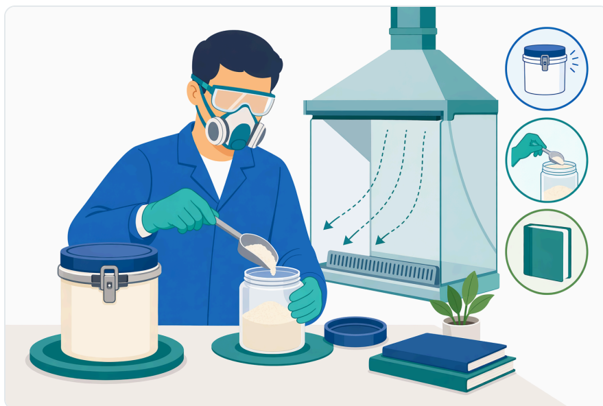
Figure 7. Powdered enzyme preparations should be handled to minimize dust exposure and unnecessary skin, eye, or inhalation contact.
